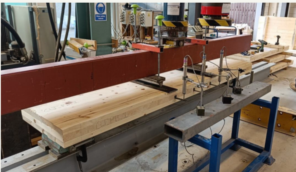
Figure 2 - 3ply CLT - Test setup for bending out-of-plane
